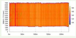
Fig. 8: Surface temperature profile with infrared camera (SBUFb, 2018).
