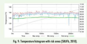
Based on the temperature profiles, risk areas are calculated that have less than 90% of the floating average value of the surface asphalt layer. A value, called PDI, is derived from these risk areas and the bonus or deduction is calculated from this PDI value with the help of a table or with specified equations (se also SBUFb, 2018; Statens vegvesen, 2019).
