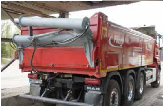
← "Wiesel" distribution screw can be simply attached / retrofitted
