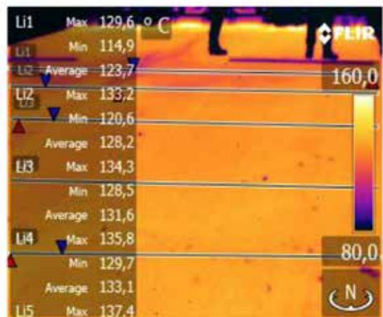
Fig. 14: Thermal image and analysis diagram of a batch from a thermally insulated dumper, incl. pusher system without feeder
